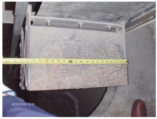
• **1910.68(b)(7)(i)***Fixed type*. On the ascending side of the manlift floor openings shall be provided with a bevel guard or cone meeting the following requirements
